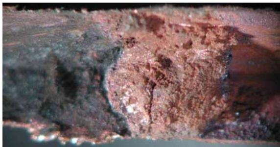
**Figure 6:** Compact oxide plug in a used hollow conductor taken from a generator.
