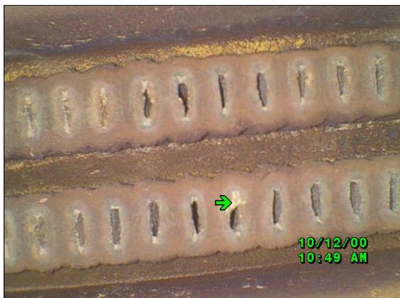
**Figure 1:** Copper oxide deposits at the hollow conductor inlet
